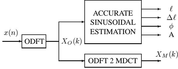
Figure 1: Sinusoidal estimation is performed in the ODFT domain which also leads to the MDCT domain.
