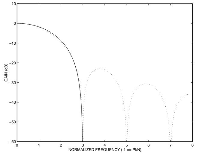
Figure 5: Normalized magnitude of the frequency response of  $|H(\omega)|$  (dotted) and simplified model of the main lobe (solid).
