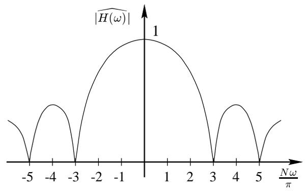
Figure 2: Normalized frequency response of the analysis window.
