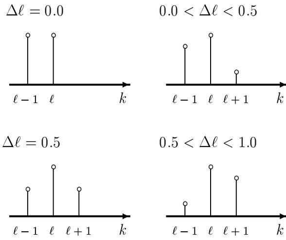
Figure 4: Relation between the magnitudes of the ODFT channels  $\ell - 1$ ,  $\ell$ , and  $\ell + 1$  when the input signal is a sinusoid whose frequency is given by  $\frac{2\pi}{N}(\ell + \Delta\ell)$ .
