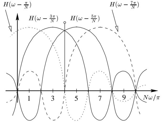
Figure 3: Illustration of the frequency responses of the first four channels of the ODFT filter bank.
