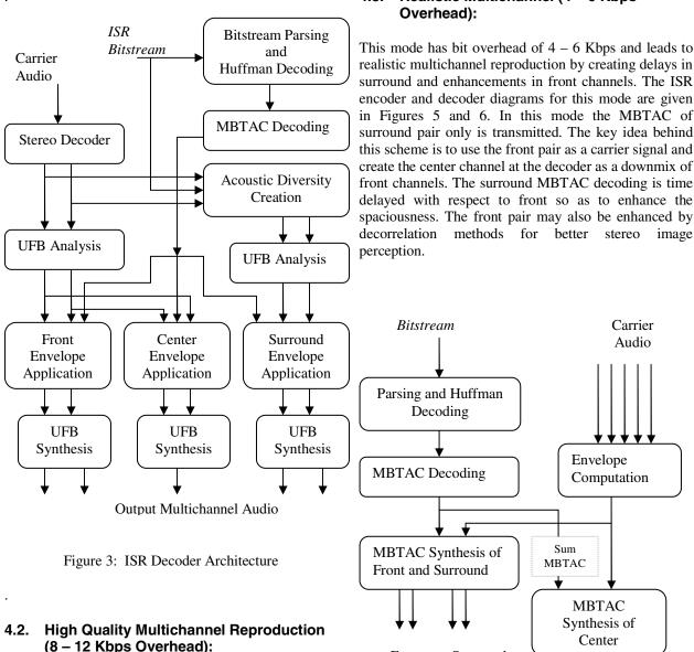
8 – 12 Kbps bit overhead is obtained by computing and transmitting the MBTAC of front and surround pair only as in Figure 4. It is assumed that the center channel is dominated by front pair and can be synthetically generating from front MBTAC. Hence instead of computing the MBTAC of center the Sum MBTAC of front pair is used on downmix of carrier audio.
