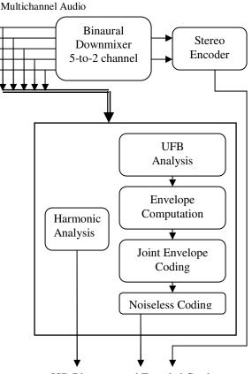
ISR Bitstream and Encoded Carrier
