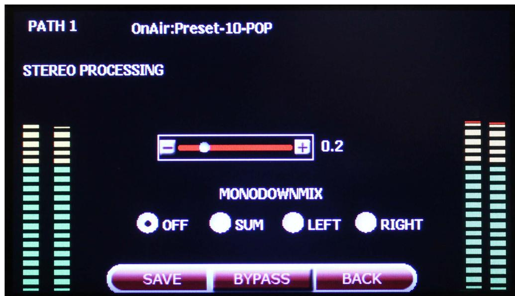
Figure 4.9: Stereo Processing
