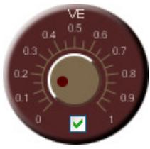
This module enhances the speech/vocal content of the audio. It uses an accurate harmonic analysis of the input audio, and effectively enhances the vocal content. Using this information input audio sounds cleaner with improved presence. This module is also useful in sports/news broadcast to make the commentators voice more intelligible, where high background audience noise exist.
