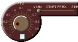
This module dynamically detects the sibilant and fricative sections of the input audio and smoothes out these sections.
