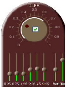
This is an audio sweetening tool that conditions the temporal envelope of the audio signal in multiple frequency bands. The 6 vertical bars below the dial provide finer control over envelope conditioning in individual frequency bands (with indicated center frequency values). The higher the sliders, the more conditioned the audio in that band is. There are two associated slider controls
